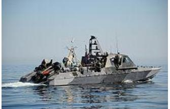
One of the US Navy's Boeing unmanned drone Mark V Special Operations Craft (SOC.)
