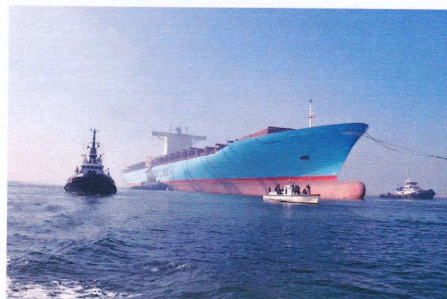
The mighty Emma Maersk being escorted from the Suez Canal in December after suffering serious leaks caused by insecure cable penetrations through an after watertight bulkhead. These were considered by her master to be potentially critical to her canal draught. She was repaired at the North Suez container terminal and sailed south two days later.
